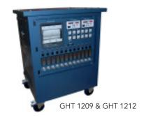
**Product:** Globe's range of 100kVA and 130kVA, twelve channel heat treatment centres, provide a complete solution for most heat treatment processes with the power transformer, switching, temperature recording and temperature profile programmer/controller instruments enclosed in a single mobile unit.
